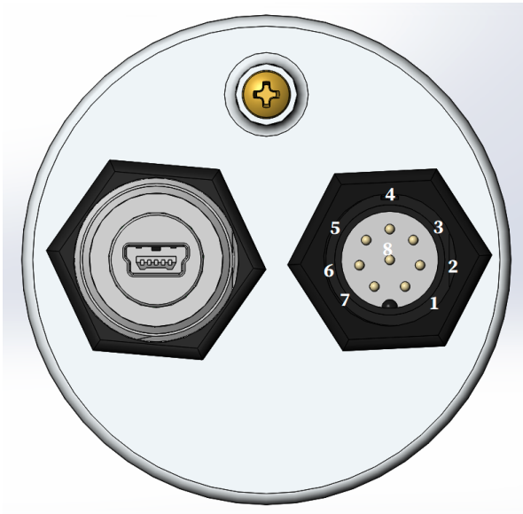
Fig. 24: Pin numbers on the EN3P8 (8-pin GPIO) connector. The SiPM-2000 board exposes the same connectors.
