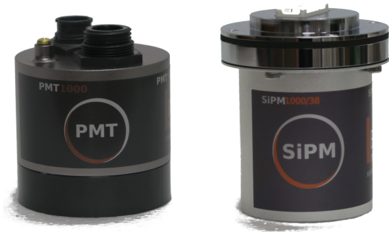
Fig. 1: Two of the many MCA-1000 variants, one for PMT and one for SiPM. PMT-1000 MCA with high voltage unit on the left. On the right: SiPM-1000 MCA+detector assembly with SiPM array and 38mm NaI(Tl) crystal in detachable housing.
