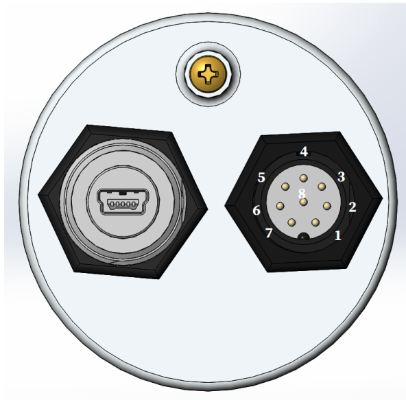
Fig. 32: Pin numbers on the EN3P8 (8-pin GPIO) connector. The connectors and pinouts are the same for the PMT-2000 and the SiPM-2000.
