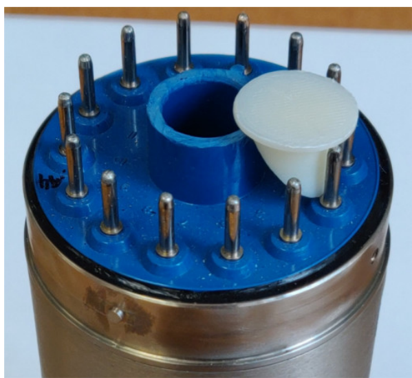
Detector with an opening for the LED. The white light diffuser is shown on the side.
